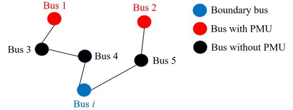
Fig. 4. Estimating phase angle of bus  $i$  using PAC.
