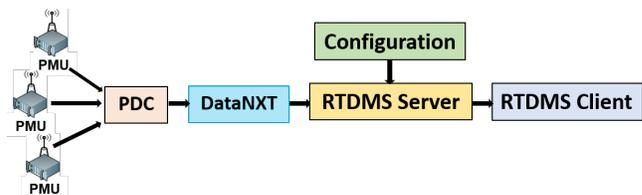
Fig. 18. Platform of real-time application of AAM.
