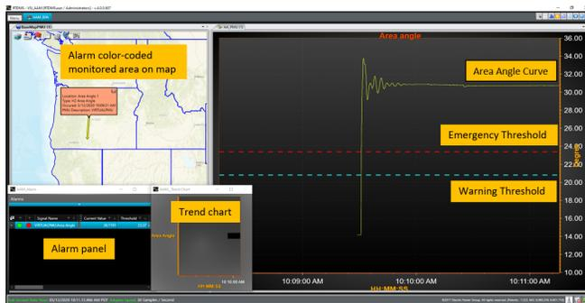
Fig. 19. Visualization of area angle in real-time.
