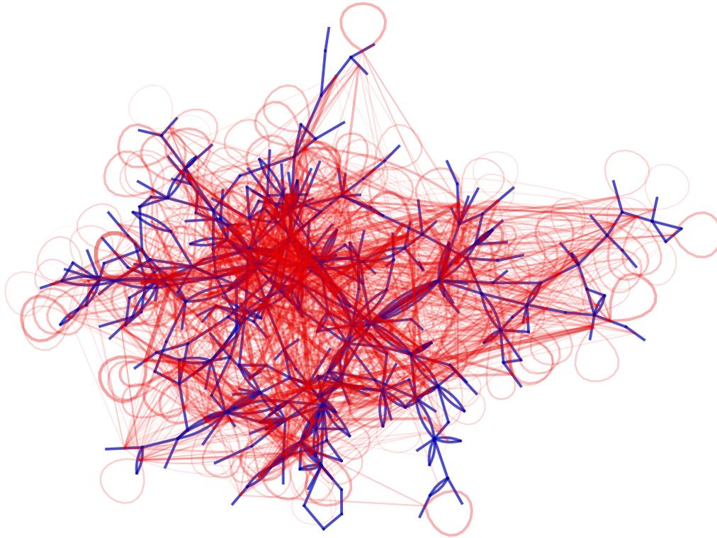
Fig. 2. The blue network is the physical utility network and the red network joining the blue lines is the influence network  $H_{1+}$  formed from the transmission line pairs in which one outage causes another. Self-loops at a node indicate lines which outage again, within the same cascade, after a time interval.
