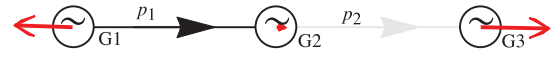
Fig. 1. The gray lines joining the buses show the magnitude of the power flow with the grayscale and the direction of the power flow with the arrows. The red arrows at each bus show the oscillation mode shape; that is, the magnitude and direction of the complex entries of the right eigenvector x associated with the interarea mode.
