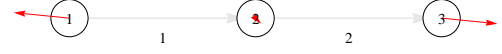
Fig. 3: The gray lines joining the buses show the magnitude of the power flow with the grayscale and the direction of the power flow with the arrows. Each line is numbered as shown. The red arrows at each bus show the oscillation mode shape; that is, the magnitude and direction of the complex entries of the right eigenvector x associated to the critical complex eigenvalue \lambda . Buses 1, 2 and 3 are generator buses.
