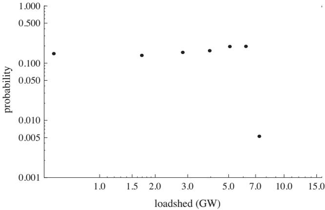
Fig. 2. Probability distribution of initial load shed by OPA on IEEE 300 bus system at load level 1.05 times the base case.
