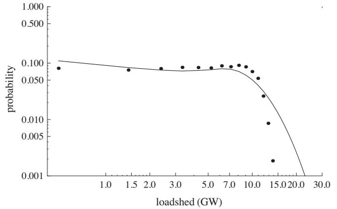
Fig. 5. Probability distributions of total load shed by OPA on IEEE 300 bus system at load level 1.1 times the base case. Dots are the empirical distribution; line is predicted with the discretized branching process.
