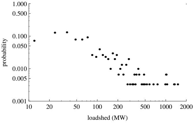
Fig. 6. Distribution of initial load shed. Data produced by TRELSS.
