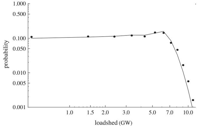
Fig. 1. Probability distributions of total load shed by OPA on IEEE 300 bus system at the base case load level. Dots are the empirical distribution; line is estimated with the branching process.
