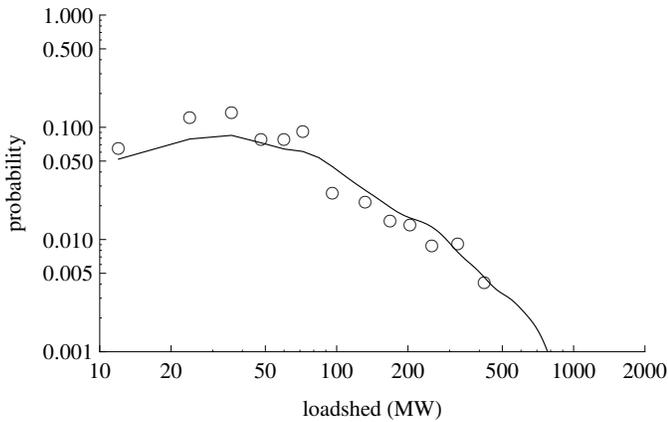
Fig. 7. Distribution of total load shed estimated by the discretized branching process (line) is compared to the binned empirical distribution of total load shed (circles). Data produced by TRELSS.
