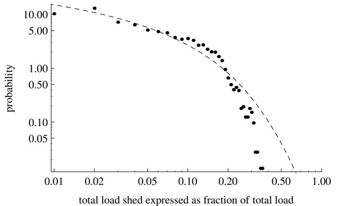
Fig. 9. Probability density function of total load shed on log-log plot. PDF estimated with continuous state branching process (dashed line) is compared to empirical PDF (dots). Empirical data from OPA on IEEE 118 bus system with the base case load level.
