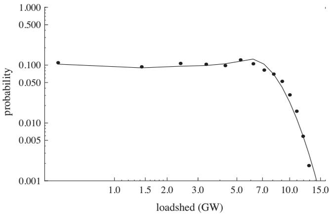
Fig. 3. Probability distributions of total load shed by OPA on IEEE 300 bus system at load level 1.05 times the base case. Dots are the empirical distribution; line is predicted with the discretized branching process.
