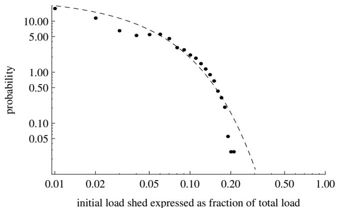
Fig. 10. Probability density function of initial load shed  $X_0$  on log-log plot. Estimated PDF (dashed line) is compared to empirical PDF (dots). Empirical data from OPA on IEEE 118 bus system with the base case load level.
