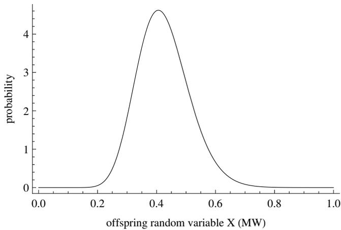
Fig. 11. Probability density function  $H(x)$  of offspring distribution that is a gamma distribution with mean  $\lambda = 0.429$  and variance  $\sigma_{\text{off}}^2 = 0.0123$ . Parameters computed from data from OPA on IEEE 118 bus system with the base case load level.
