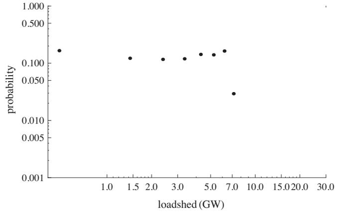
Fig. 4. Probability distribution of initial load shed by OPA on IEEE 300 bus system at load level 1.1 times the base case.
