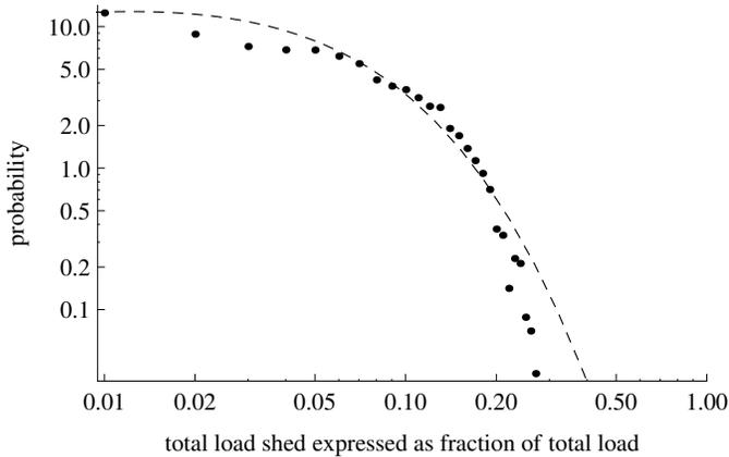
Fig. 8. Probability density function of total load shed on log-log plot. PDF estimated with continuous state branching process (dashed line) is compared to empirical PDF (dots). Empirical data from OPA on IEEE 118 bus system with load level 0.85 times the base case.
