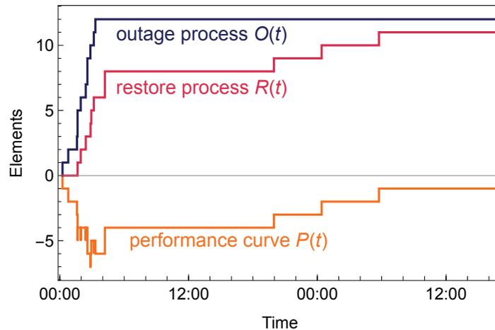
**Fig. 6** Processes for a transmission system event with 12 outages. Image from [9] is licensed under CC BY 4.0.
