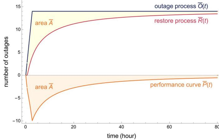
**Fig. 7** Typical North American transmission system resilience event tracked by number of outages on the vertical scale. The shaded area  $\bar{A}$  of  $\bar{P}(t)$  is a useful metric and is the same as the shaded area between  $\bar{O}(t)$  and  $\bar{R}(t)$ . Image from [55] is licensed under CC BY 4.0.
