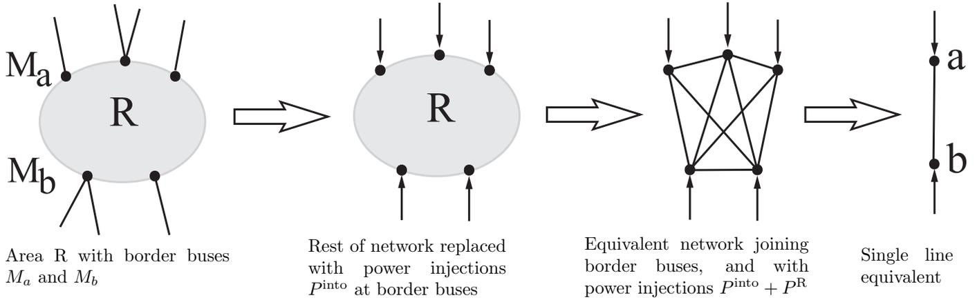
Fig. 1: Reduction of area R to a single line equivalent that describes the electrical characteristics between the set of border buses  $M_a$  and the set of border buses  $M_b$ . Angle across area R from  $M_a$  to  $M_b$  is the angle  $\hat{\theta}_{ab}$  across the single line from  $a$  to  $b$ . Power flow through area R from  $M_a$  to  $M_b$  is the single line power flow  $P_{ab}$ . Area R susceptance is the single line susceptance  $b_{ab}$ .
