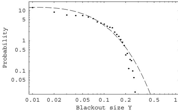
Fig. 8: IEEE 118 bus system with loading factor 0.85. Probability density function of fraction of load shed  $Y$ . PDF estimated from branching process (dashed line) compared with empirical PDF from OPA simulation (dots).
