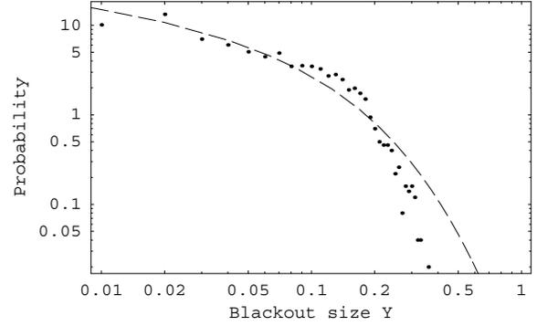
Fig. 9: IEEE 118 bus system with loading factor 1.0. Probability density function of fraction of load shed  $Y$ . PDF estimated from branching process (dashed line) compared with empirical PDF from OPA simulation (dots).
