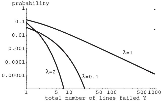
Fig. 2: Probability distributions of total number of line failures  $Y$  according to the generalized Poisson distribution with saturation at  $S = 1000$  lines for three values of propagation  $\lambda$ . The distribution has an approximate power law region at criticality when  $\lambda = 1$ . The probability of 1000 lines failing is 0.025 for  $\lambda = 1$ , and 0.797 for the supercritical case  $\lambda = 2$ .
